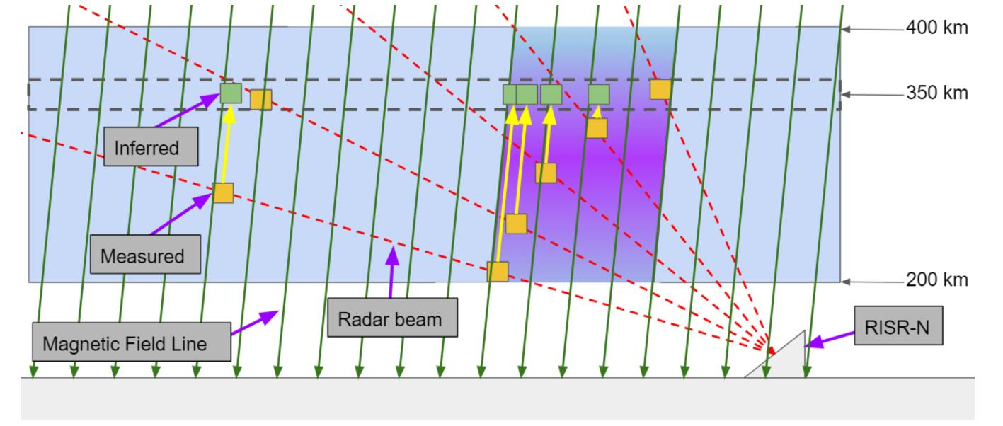
**Figure 3**: The field-line mapping technique used to infer plasma densities at 350 km in the presence of a plasma structure (shown in purple). The red lines are radar lines-of-sights, the orange squares are positions measured, the green squares are inferred measurements, and the green arrows are magnetic field-lines.
