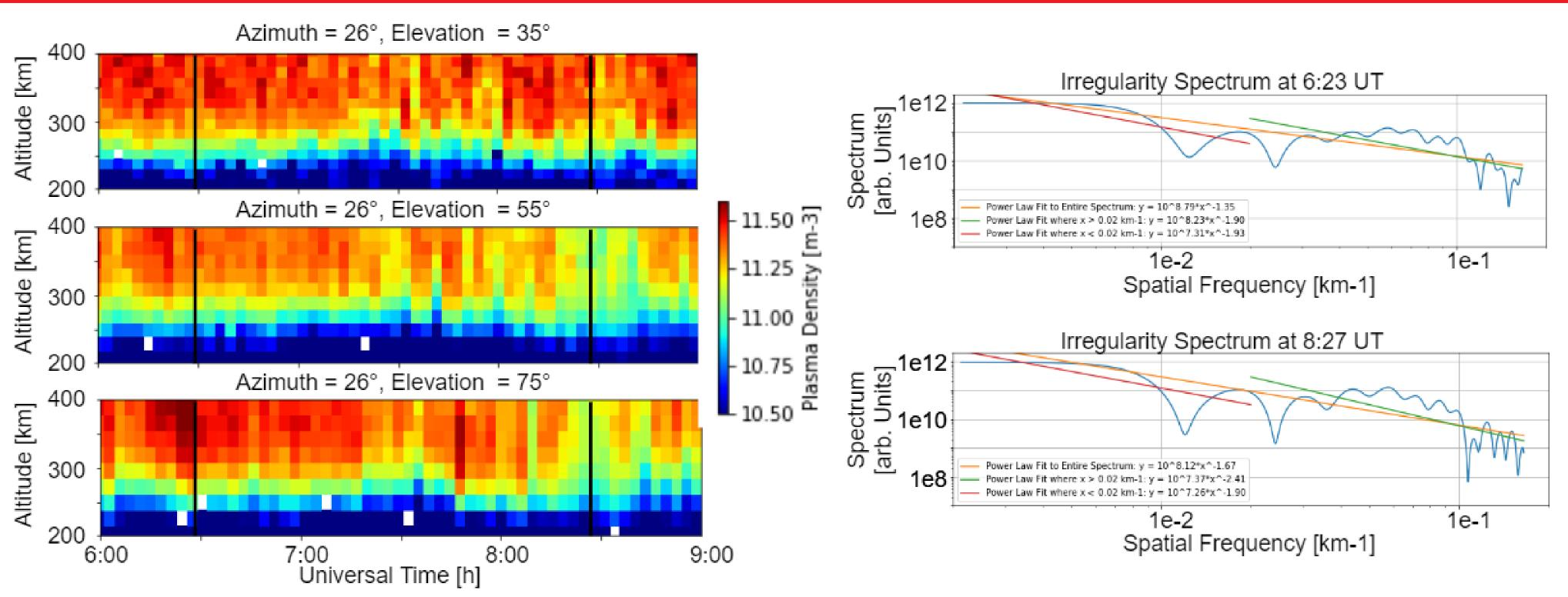
Figure 1: a) Chatanika ISR. b) Midnight auroral zone Chatanika ISR plasma density observations (contour interval is 2e4 cm-3). c) Associated irregularity spectrum developed using observations at 350 km altitude [Kelley et al., 1982].
